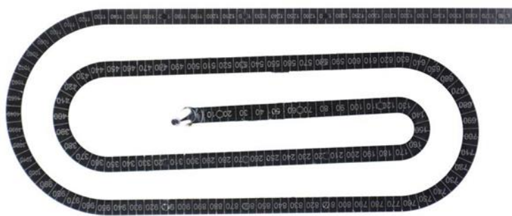
Figure 17. PF6680 (GF25+GB30) and PF1110 (GF35+GB45); the spiral molded part
